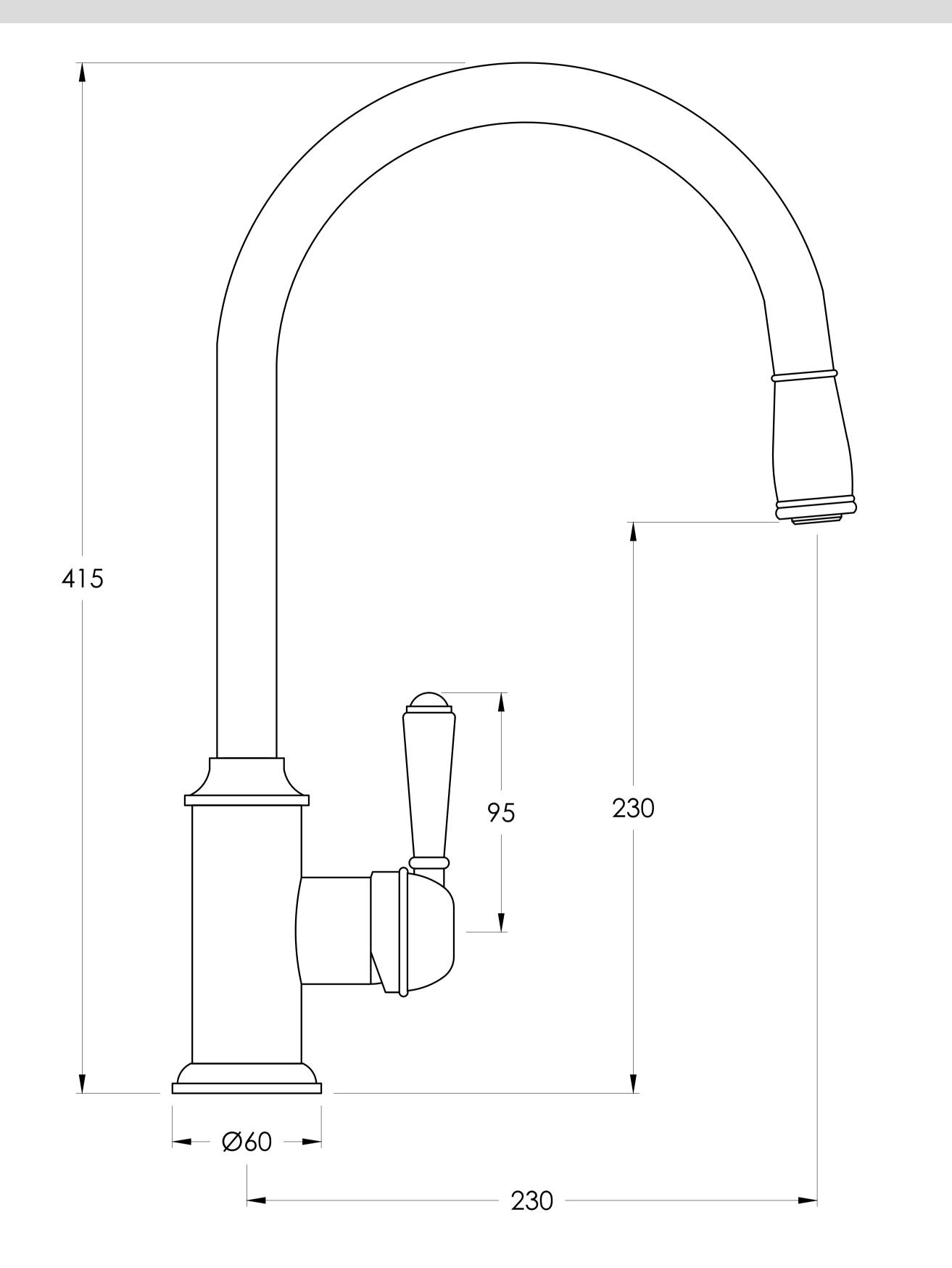
Note: Mixer requires a Ø35mm hole in the bench or basin Max benchtop thickness of 28mm
