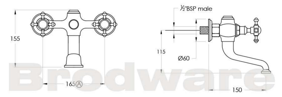
Note: G½" BSP female fittings required in the wall A Fixed centre; outlets must have 165mm centres
