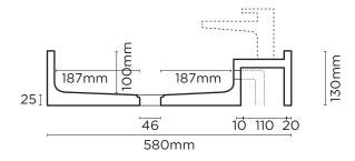
Note: Overflow pipe separate. For surface mount basin, a second hole in bench top is required.
