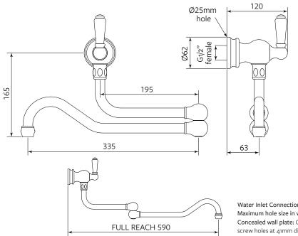
Water Inlet Connection: 15mm Maximum hole size in wall: Ø25mm Concealed wall plate: Circular with 4 screw holes at 41mm diagonal spacing
