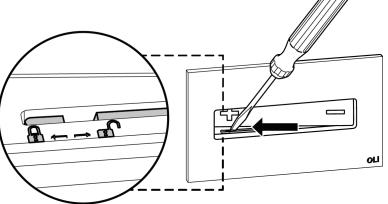
This push plate uses a "Segull wing" opening, which allows an easy opening and prevents from falls and damages during installation and maintenance.
