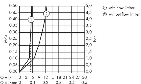
**AXOR Citterio****3-hole basin mixer for concealed installation wall-mounted with spout 162 mm, cross handles and escutcheons**
