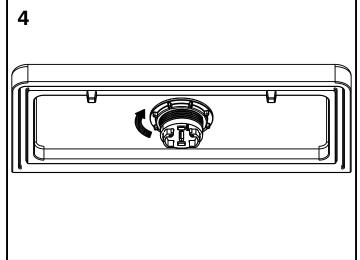
Hand tighten the nut fully.
