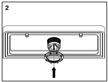
Screw the nut on the button assembly from underneath the lid.
