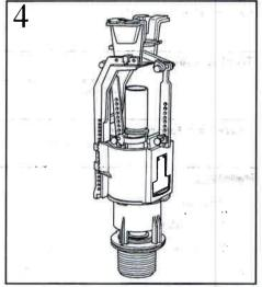
Attach old button assembly to new valve.
