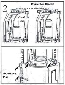
Remove old valve and place next to new valve on flat surface. Set height of the connection bracket by adjusting position of pins & cut Overflow Tube to match old valve. NOTE: This is critical to ensure Air Separation is maintained between the Overflow Tube and the Inlet Valve
