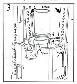
Ensure yoke sits approximately 3mm under overflow tube. Trim off excess lifter lengths.
