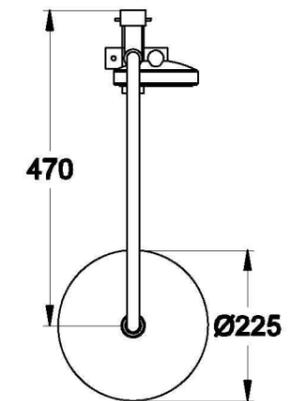
Note: top inlet feed required 1/2 inch BSP male thread in wall
