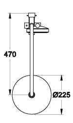
Note: top inlet feed required 1/2 inch BSP male thread in wall
