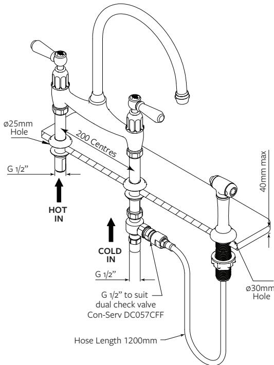
**Please Note:** This model does not suit incoming water pressure below 100kPa or higher than 500kPa. The spray rinse model requires a minimum inlet pressure of 100kPa to successfully divert the water flow from the main tap to the spray rinse. The stop cocks provided with this tap contain gauze filters. Please ensure your plumber is advised of the minimum and maximum water pressure, and to install the stop cocks as failure to do so voids the tap warranty.
