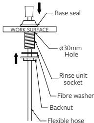
Secure the rinse unit socket in a suitable position using a tap wrench of a 36 AF spanner.
