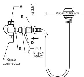
Ensure the black rubber washers are situated inside positions A, B, C, F and E on the rinse connector, including the double check non-return valve as shown in the diagram.
