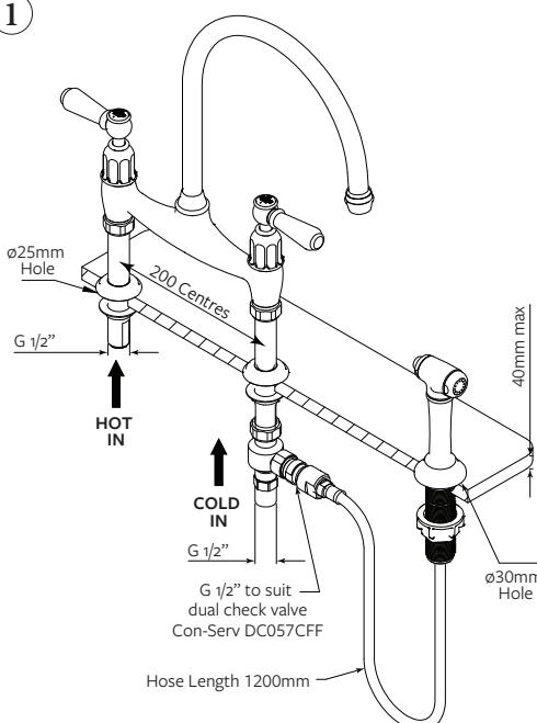
Ensure the mixer is oriented correctly, levers should rotate to point forward and the hot index should be situated on the left.
