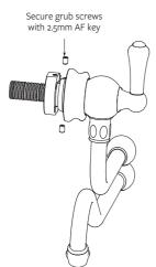
Slide the rosette forward to access the retaining screws.
