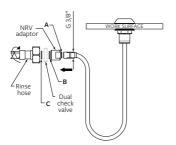
Ensure the black rubber washers are situated inside position A, B (either side of NRV) and C on the rinse hose, including the NRV adaptor in sequence as displayed in the diagram.
