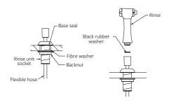
Thread the tapered end of the rinse flex hose into the rinse unit, ensuring the rubber seal is in place between them.
