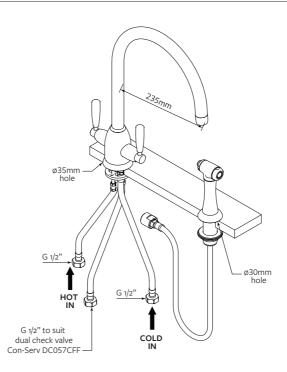
Please Note: This model does not suit incoming water pressure below 100kPa or higher than 500kPa. The spray rinse model requires a minimum inlet pressure of 100kPa to successfully divert the water flow from the main tap to the spray rinse. The stop cocks provided with this tap contain gauze filters. Please ensure your plumber is advised of the minimum and maximum water pressure, and to install the stop cocks as failure to do so voids the tap warranty.
