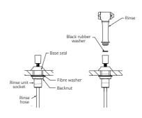
Thread the tapered end of the rinse flex hose into the rinse unit, ensuring the rubber seal is in place between them.
