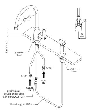
Please Note: This model does not suit incoming water pressure below 100kPa or higher than 500kPa. The spray rinse model requires a minimum inlet pressure of 100kPa to successfully divert the water flow from the main tap to the spray rinse. The stop cocks provided with this tap contain gauze filters. Please ensure your plumber is advised of the minimum and maximum water pressure, and to install the stop cocks as failure to do so voids the tap warranty.
