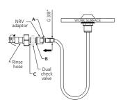
Ensure the black rubber washers are situated inside position A, B (either side of) and C on the rinse hose, including the NRV adaptor in sequence as displayed in the diagram.
