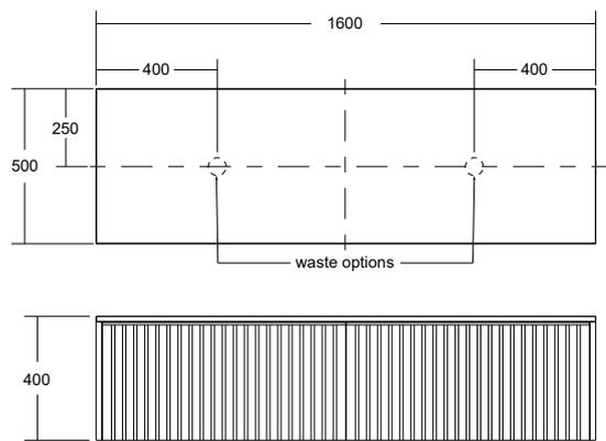
\* Height indicated on the drawing is for the cabinet with a timber bench top. The height with solid surface bench top is 394mm.
