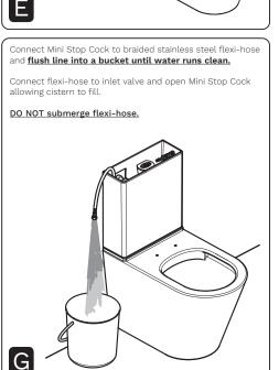
Back Inlet installation install the Mini Stop tap to wall outlet.
