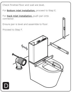
Bottom Inlet installation, attach mini stop tap to the wall outlet. Connect the flexi-hose to mini stop tap.
