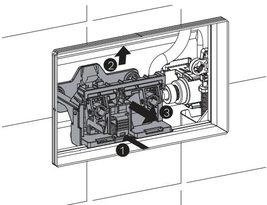
10 Turn off mini stop valve &amp; unhook fill valve from the clip
