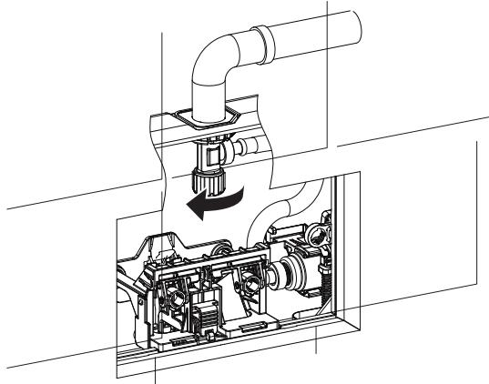
Open mini stop valve and check for leaks
