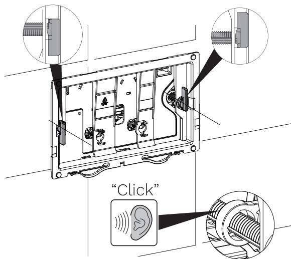
32 Make sure the length of adjustable rod is adequate and have no interference
