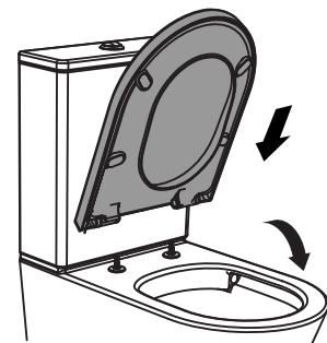
4 Adjust seat position so that front of seat is forward to toilet pan by 2-3mm.
