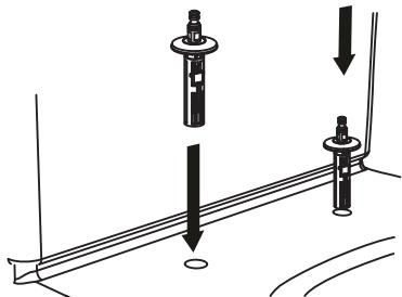
2 Using the spanner tool supplied, screw in hinge pins. Do not over tighten so as to allow adjustability.
